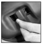
To tilt the wheel, first pull the lever towards you release the lock. Then move the steering wheel to a comfortable level, and release the lever to lock the wheel in place.
